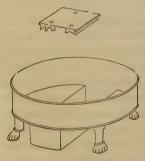
but never with advantage, because of their complexity of form, and the consequent difficulty of keeping the numerous joints tight. They are often on a smaller scale, and when the chemical establishment altogether is small, are then more in proportion to the rest of the apparatus. A very useful table trough is of a circular form, and about two feet in diameter, internally divided into
